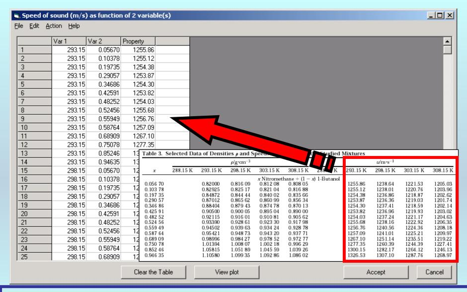
**NOTE:** Simple CUT/PASTE procedures can be used within the table to convert the original table into the required number of columns. (This can also be done externally in spreadsheet software, e.g., EXCEL.)
