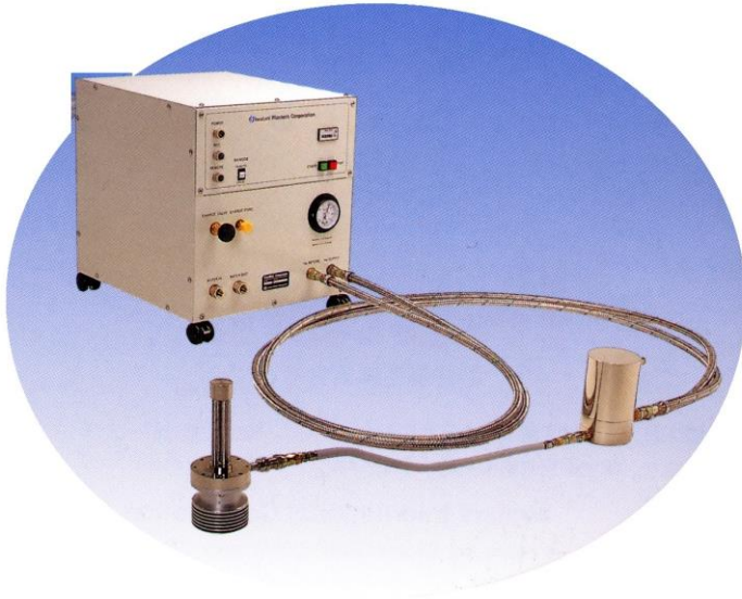
Figure F1.13. First commercial pulse tube cryocooler, showing Gifford-McMahon compressor and rotary valve.
