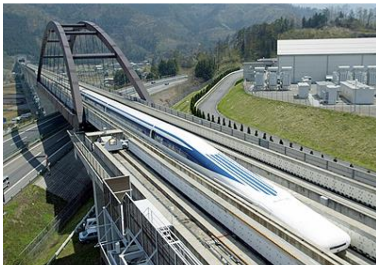
Figure 19: Japanese Maglev train that uses superconducting magnets for levitation and has a rated speed of 500 km/hr. Image: Central Japan Railway Company
