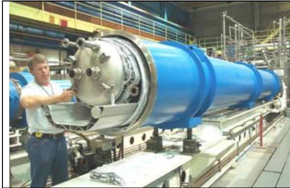
Figure 17: One dipole magnet being assembled into a cryostat for the LHC at CERN. The two tubes near the center are the two beam tubes. Image: CERN.
