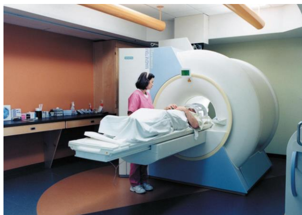
Figure 14: Modern MRI system with a 1.5 T superconducting magnet and cryocooler.
