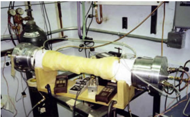
Fig. 36. CSIR straight-prototype during testing at LANL using two of the SETAC drivers attached at either end [100].
