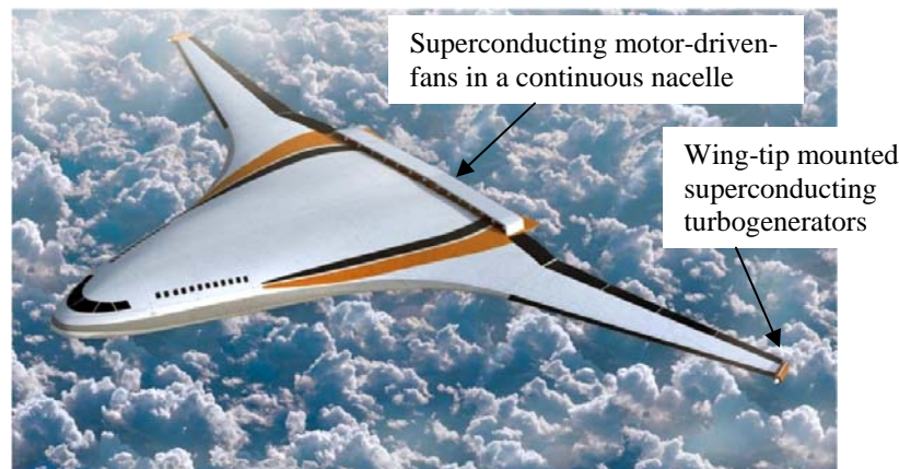
FIGURE 1. Artist's concept of future turboelectric aircraft utilizing superconducting generators and motors [2].
