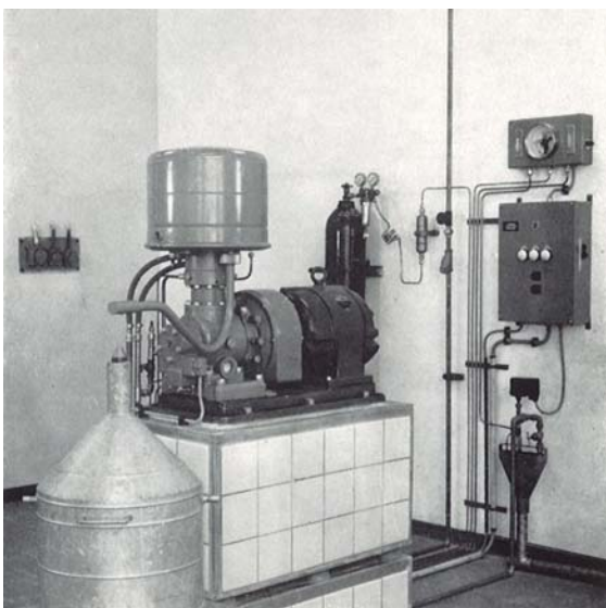
Figure 15. First commercial Philips air liquefier. (A-machine) Kohler (1960).
