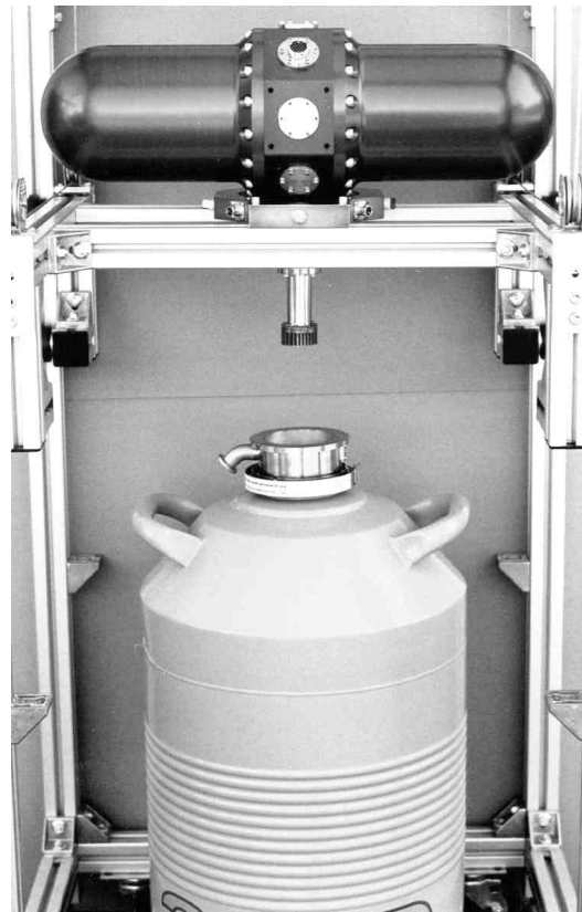
Figure 1. Pulse tube liquefier system.
