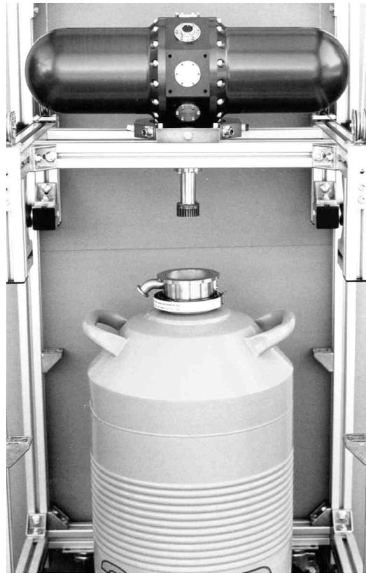
**Figure 1.** Pulse tube liquefier system.
