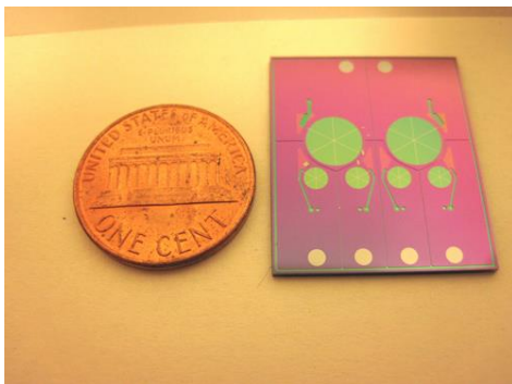
FIGURE 5. Two-stage chip-scale vacuum micropump developed by MIT. Courtesy of DARPA.
