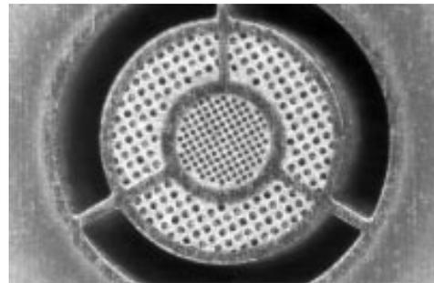
**Figure 8.** End view of heat exchanger. The top layer is a stainless steel spacer and the copper perforated plate can also be seen.
