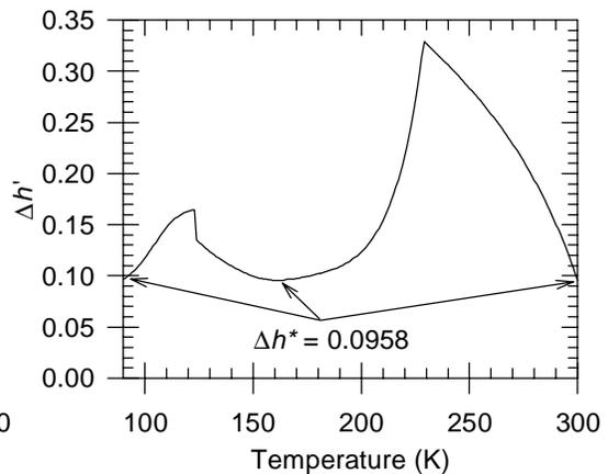
**Figure 5.** Normalized enthalpy for 38.5% nitrogen, 27.5% methane, 10.5% ethane, and 23.5% isobutane.
