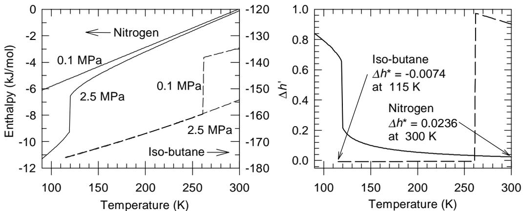
Figure 2. Enthalpy and normalized enthalpy for nitrogen and iso-butane.
