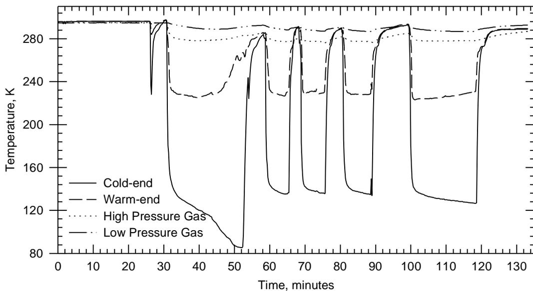
**Figure 9.** Catheter test results. The cold end is the catheter tip, the warm end is on the surface of the outer lumen at the warm end of the heat exchanger, high pressure gas is the gas temperature entering the inner lumen, and the low pressure gas is the gas temperature leaving the outer lumen.
