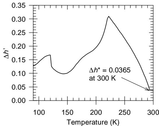
**Figure 4.** Normalized enthalpy for 45% nitrogen, 20% methane, 20% ethane, and 15% isobutane.
