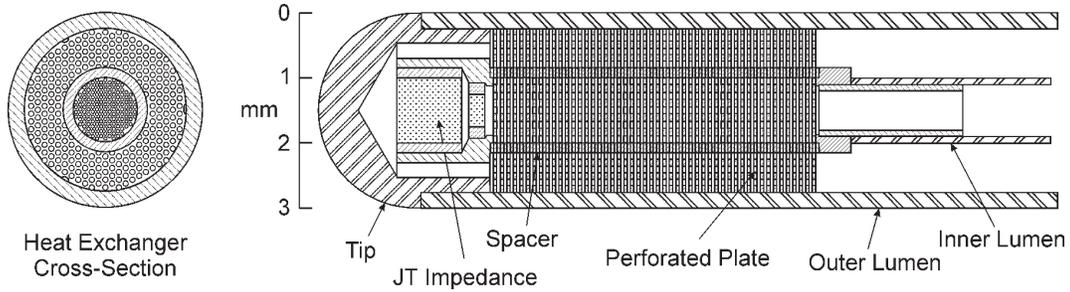
**Figure 6.** Schematic diagram of catheter tip.
