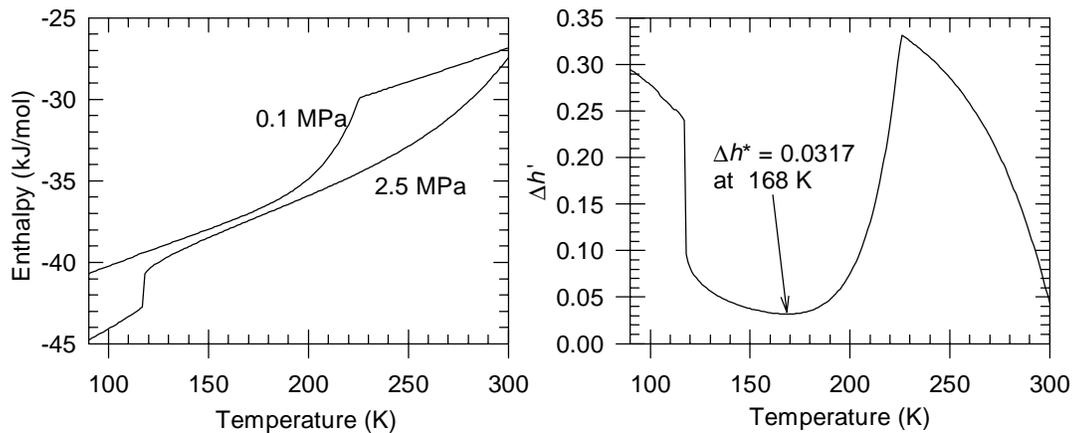
Figure 3. Enthalpy and normalized enthalpy for 80% nitrogen and 20% iso-butane.
