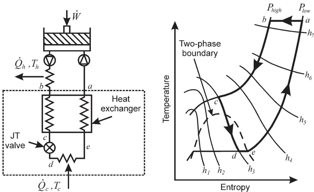
Figure 1. Schematic diagram of a Joule-Thomson system with temperature-entropy diagram.
