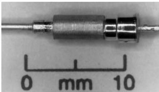
**Figure 7.** Catheter cold end. The tube on the right is only for making pressure measurements and is not part of the working catheter. The left tube is the high pressure inlet to the heat exchanger.
