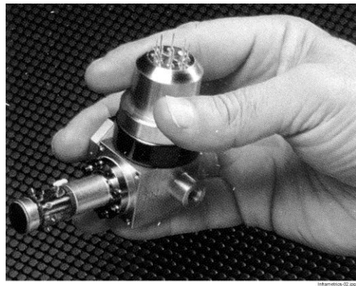
Figure 8. Stirling micro cryocooler that provides 0.15 W of cooling at 80 K with 3 W of input power. Courtesy Inframetrics/FLIR Systems.
