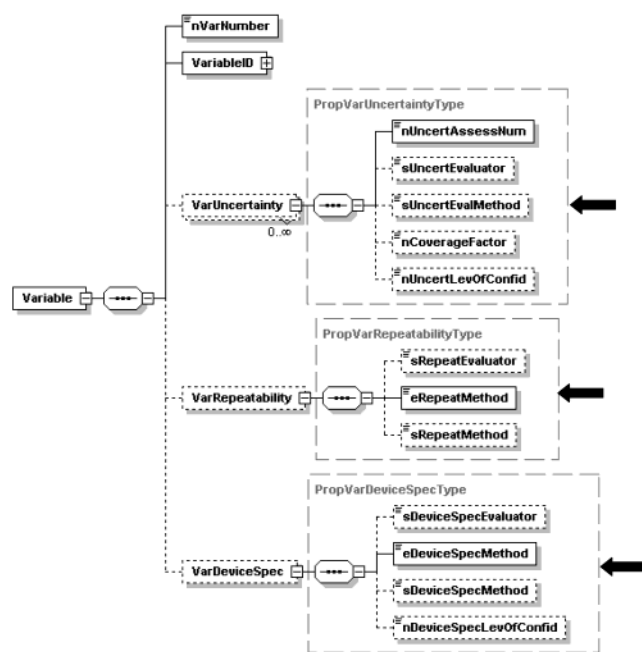
Figure 9. Structure of the Variable element in the “ ReactionData ” block. The arrows indicate new elements described in the text.
